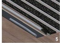
Continue the process until the last profile and adjust **Basmat** in the mat well. Insert the foam tubes under the initial and final wings.
