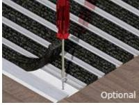
Screw **Basmat** to the floor. Stick the finish strips to the aluminium profiles.
