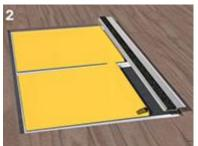
Place the self-adhesive black foam strips parallelly to each other with the adhesive part facing upwards. Peel off the protective paper a few centimeters. The exterior foam strips must be at a distance between 2-5 cm from the edge. The profile with the **Basmat** label must be the last one to be installed.
