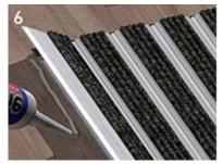
Fix **Basmat** to the floor with adhesive or silicone. If desired, **Basmat** can be screwed to the floor (see Optional section).
